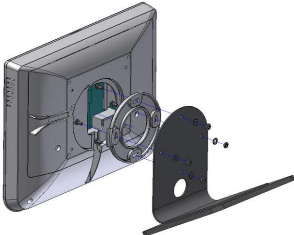
Screw for mounting the base on the frame
